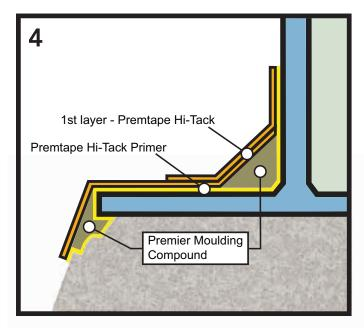
Apply the first strip of PREMTAPE HI-TACK™ in line with the masking tape starting from the concrete base. Subsequent strips should overlap each other by a minimum of 50mm with the final strip applied in line with the masking tape on the vertical face. Smooth down all layers of tape ensuring there are no air pockets.
