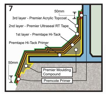
Brush apply 2 coats of the PREMIER™ ACRYLIC TOPCOAT onto the PREMIER ULTRASEAL RT TAPE. To ensure that the wider-interleaving edges of Premier Ultraseal RT Tape are coated and completely wet through with the final layer of ACRYLIC TOPCOAT, we recommend that masking tape is applied 15mm above the wider interleaving edge of ULTRASEAL RT Tape.
