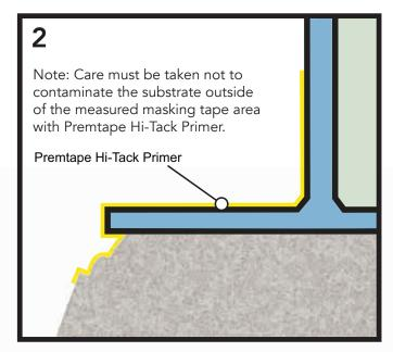
Measure, mask (50mm width masking tape) and prime the area for PREMTAPE HI-TACK $^{\text{TM}}$ .
