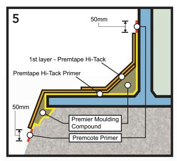
Measure and mask top and bottom allowing for the application of a 50mm strip of PREMCOTE™ PRIMER as shown in red. Brush apply primer and allow to dry (approx 20 minutes). Now remove second two strips of 50mm width masking tape from top and bottom of application area.
