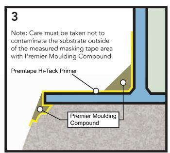
Fill all small voids, cracks and profile the 90° Tank Base angle with a 45° fillet of PREMIER™ MOULDING COMPOUND.
