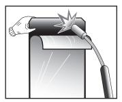
Peel back about 200mm of release liner from the trimmed end of the sleeve. Gently heat exposed adhesive.
